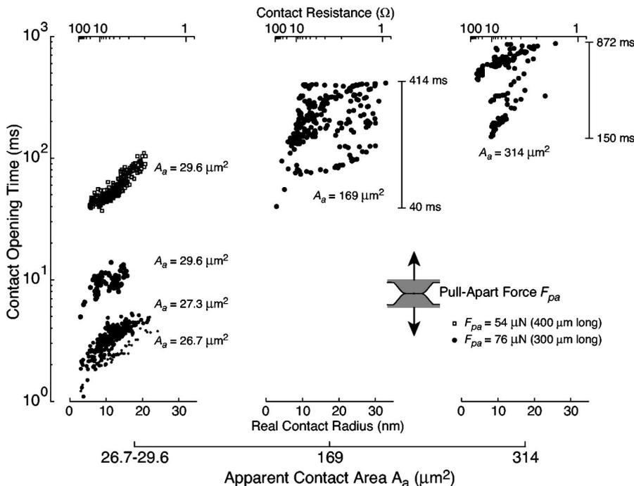
FIG. 4. Switch opening time data for all switches showing dependence on real contact radius, apparent contact area, and pull-apart force.
