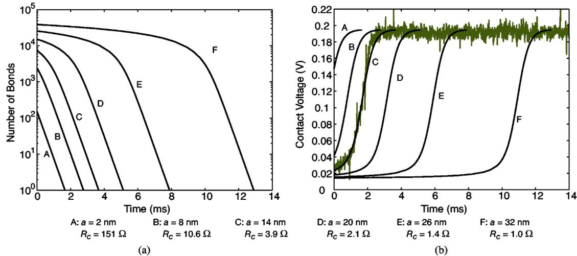
FIG. 7. (a) Sample solution curves to Eq. (10) with  $A_a = 27.3 \mu\text{m}^2$  and (b) corresponding contact voltage plotted with the measured data of Fig. 3. Solutions are shown for various values of the real contact radius  $a$  and the corresponding initial contact resistance  $R_c$  (or resistance before opening begins).
