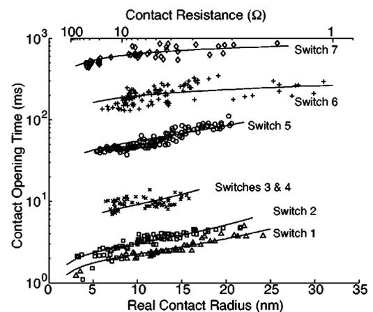
FIG. 8. Comparison of the model to the data at a contact force of 66– $76 \mu\text{N}$ .
