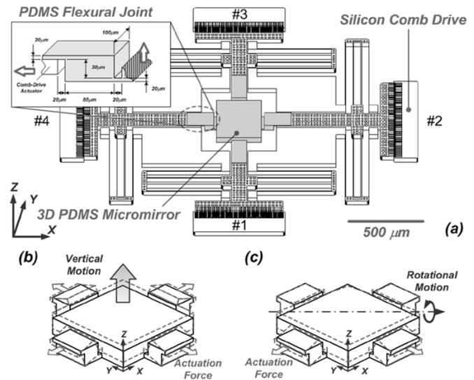
Fig. 1. (a) Schematic drawing of polymer-based scanning micromirror with single-layer silicon comb drives. (b) Vertical motion of micromirror. (c) Rotational motion of micromirror.
