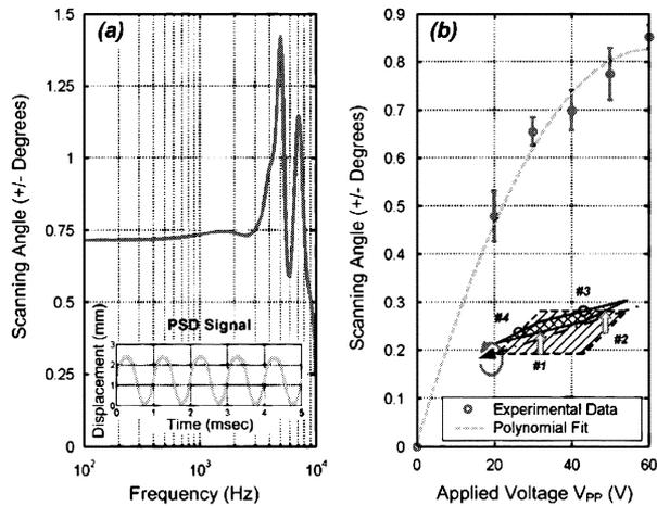
Fig. 4. Experimental results of rotational motion measurement. (a) Frequency response of micromirror rotational motion. The figure inset shows positional signal detected using the PSD at a sinusoidal actuation voltage of 1 kHz. (b) Static scanning mirror rotational angle estimated from the experimental results at 1 kHz as a function of actuation voltage.
