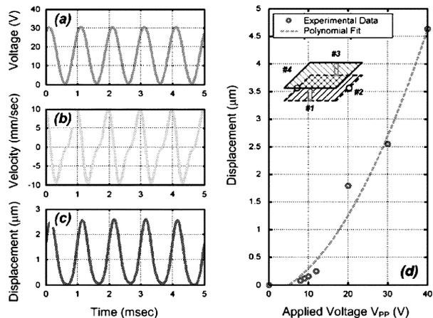
Fig. 3. Vibrometry results of vertical motion measurement. (a) Voltage signal applied on comb drives. (b) Velocity signal detected by laser vibrometer. (c) Calculated vertical displacement of mirror by integrating detected velocity signal. (d) Measured vertical motion of mirror corresponding to voltage applied on comb drives at 1 kHz.
