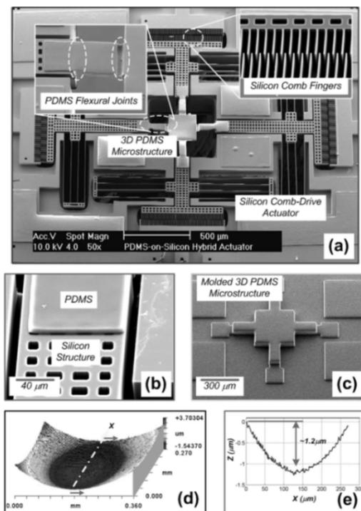
Fig. 2. Fabricated scanning micromirror. (a) SEM images of entire device. (b) Bonding interface between PDMS and silicon. (c) Molded 3-D PDMS microstructure by soft lithography. (d) and (e) Optical interferometric profile measurement results of mirror surface.
